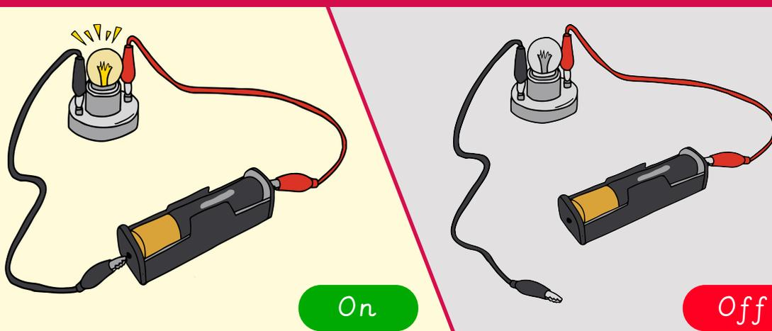
If there is a break in a series circuit, the electrical current will be cut and all the components will stop working. Causing a break in a series circuit can act as a switch to turn the circuit off.
